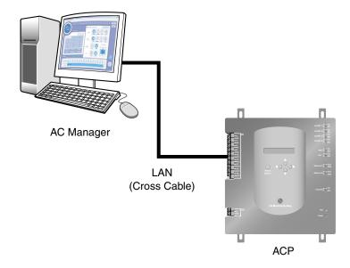
Figure. Cross cable Enlarged figure of ACP Ethernet terminal is as shown below.
