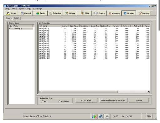
Above details reflect the air conditioner information being operated in the default control in real time. Let's find out the menu on above screen.
