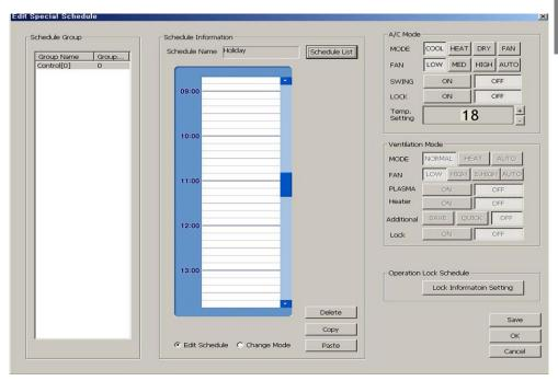
Drag time on the desired date and set the desired mode, wind strength, wind direction, temperature, all lock and etc. from air conditioner. Get the mouse off and them the setting appears in the schedule window.
