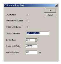
After setting, click OK to exit this window. The outdoor unit that isn't installed can be deleted using (4) Delete button in the default screen.
