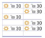
The figure on the right is an image that appears in case of heating, deactivating lock and 30°C setting.
