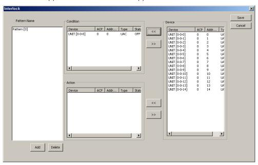
Indicate its status On when fire is detected in DI of port5-1, reflected in (3). The status of DI can be determined to be On or Off by double-clicking the device. In this case, the air conditioner connected to ACP5 should be Off as responsive action. Select air conditioner for the responsive action in (2) and click << button to reflect it to (4) action area. Now, the screen appears as below.
