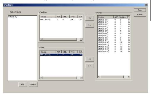
**3.** Now, set the operation status of air conditioner corresponding to the responsive print-out for the condition. Double-click the device reflected in (4) and below window appears.
