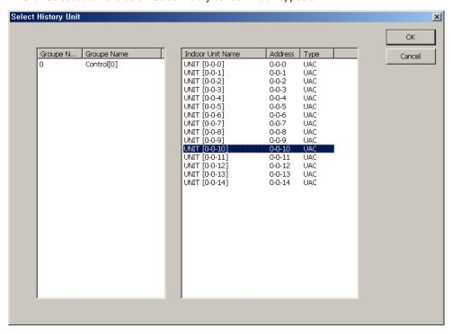
Select the desired device on above screen and click OK button. The settings are determined and the window is closed.
