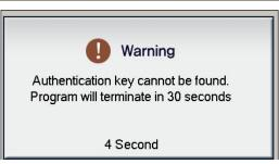
If the authentication key comes out or the user takes it out, the warning message below appears. If you insert the authentication key within 30 seconds, the warning window disappear, the program will normally operate.
