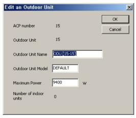
After setting, click OK button and exit this window. The outdoor unit that isn't installed can be deleted using (4) Delete button in the default screen.
