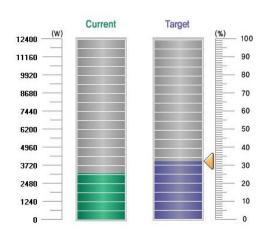
The graph indicating current operation status exists. With this graph, the facility manager can check the power value and the goal power value set when 100% of currently installed air conditioners are operated.
