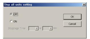
As a default, this function is checked as Deactivate. If you check Activate, you can stop the air conditioner operation for certain period. This is a convenient function when controlling the air conditioner at a time. After setting, click OK button.
