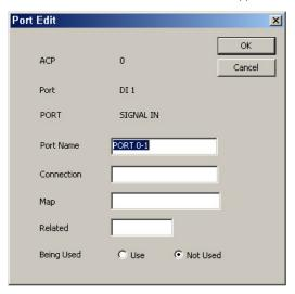
Set port name, connection device, drawing information, connected port, use and etc. and then, click OK button to save the contents.
