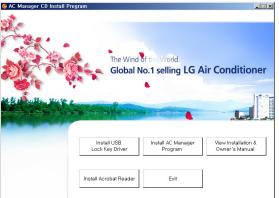
he order of menu as shown in this figure, user will install lock key driver and then AC Manager program. In this screen, you can read installation/user's manual and install Acrobat Reader program to check the manual. If you complete the installation, press Exit button.
