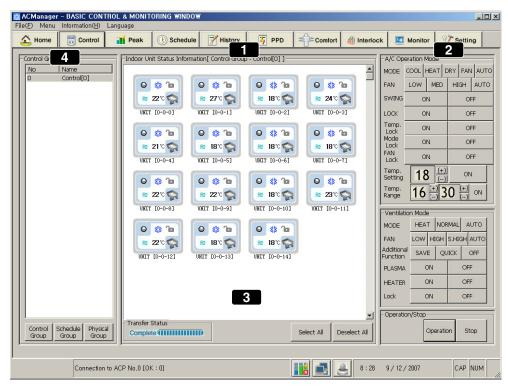
Above menu is the control program with central control method which manages the air conditioner using computer screen. Using above buttons, you can easily operate and monitor the status of air conditioner and integrately maintain the groups.
