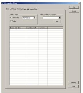
You can inquire total using time of air conditioner and using time of specific air conditioner per date respectively. Click Initialize operation time button, and you can initialize previous using time and accumulate the period again.
