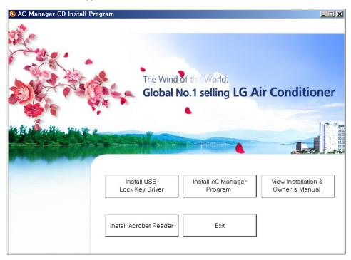
Like the order of buttons on the right, the user will install AC manager program after installing lock key driver. In this screen, you can see installation/user manual and install Acrobat Reader program in order to check the manual. If you want to exit the installation, please press exit button.
