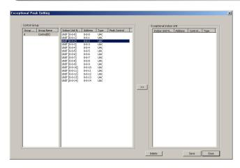
The air conditioner not to be affected by peak operation rate control can be registered. Click peak not applied button and this window appears.
