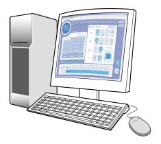
Insert Hard Lock key into USB port of AC Manager PC. All functions of AC Manager will be determined by the authentication key.
